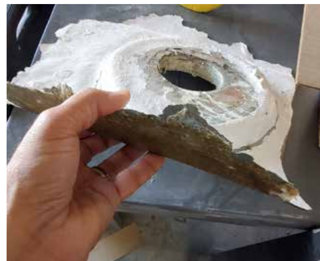
(8) Polyester resin does not bond reliably to cured polyester. This part popped loose from the hull due to a failed bond, as a result of a poor resin choice and poor preparation.
