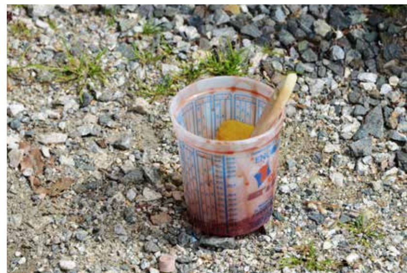
(4) A common boatyard sight: excess resin in a cup left outside overnight. A container with catalyzed resin can generate enough heat to start a fire and for that reason we always leave them outside of the shops overnight. In the morning, before tossing it away, check to make sure the resin cured properly.
