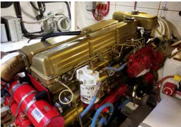
Here's a benchmark that shows the right stuff. This 30-plus year-old Ford Lehman has been well cared for by professional delivery captains Wendy and Jerry Taylor, proving that age and hours don't necessarily lead to leaks and rust.
