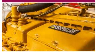
Low engine hours potentially bode well for engine longevity, provided the boat has been maintained well and run primarily at the rated recreational performance load. Engine brand and model matters; some engines have been designed for relatively low hours between rebuilds (6,000 hours, for example), while others have been engineered for much higher spans (10,000 hours, for example).
