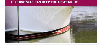
Boats with hard chines or low spray rails form a wedge-shaped pocket at the waterline near the bow. At anchor with even a minor chop, the wavelets hit this wedge and make a slap or chunk sound. You not only hear this happen; you often can feel it.
