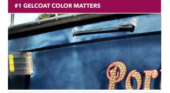
Gelcoat is a thin, pigmented, resin-rich coating on the outside of the boat. Gelcoat has two functions: to keep the water out of the fiberglass laminate, and to make the boat look pretty. The latter function explains the reason for so many hulls in dark colors such as blue, black, red and forest green.
