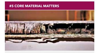
If you are buying a composite (fiberglass) boat, then you can count on two things: the hull and/or deck will have core material between fiberglass skins, and there will be elevated moisture found somewhere during the survey.
