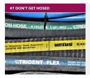
Cruising boats have a surprising amount of hose. A 40-foot trawler might have 200 or 300 feet or more of fuel, sanitation, engine, hydraulic and seacock hoses. Fuel fill hose costs roughly \$20 per foot, while good sanitation hose will come closer to \$30 per foot. And replacing hoses can be shockingly time consuming. Just imagine the run of sanitation hose from a tank in the bilge through cabinetry and up to the deck.
